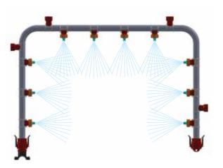
NOTE: THIS RISER CONFIGURATION AS SHOWN CONSISTS OF (2) IDENTICAL RISER SECTIONS, SHARING A SIDE-CENTRALLY LOCATED HEADER. (ONLY ONE RISER IS SHOWN FOR CLARITY.)
